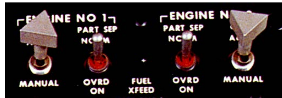
Figure 7-53 Particle Separator Switches
